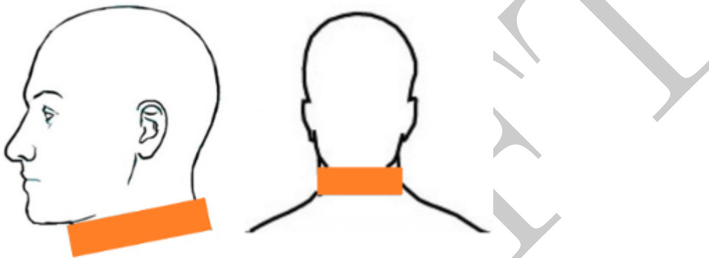
Figure 2. Areas of the neck and throat that must be protected by rigid material.
