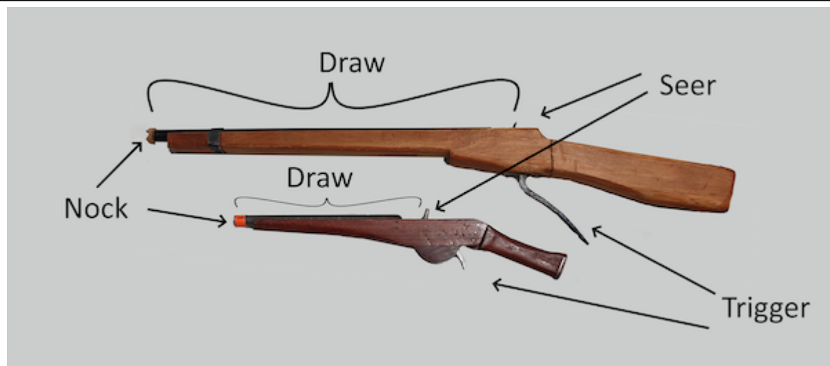
Figure 5. Draw length of a rubber band gun.
