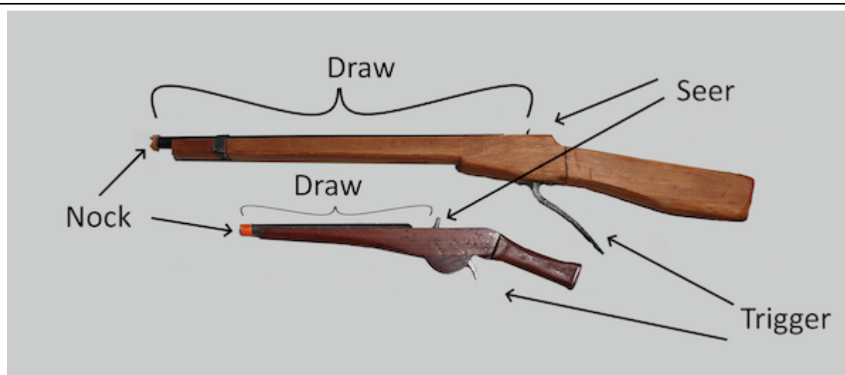
Figure 5. Draw length of a rubber band gun.
