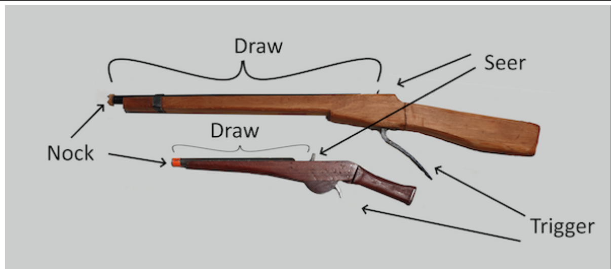
Figure 5. Draw length of a rubber band gun.
