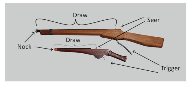
Figure 7. Draw length of a rubber band gun
